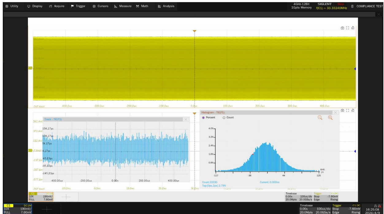
Figure 5-7 Waveform details for transmitter timing jitter test
