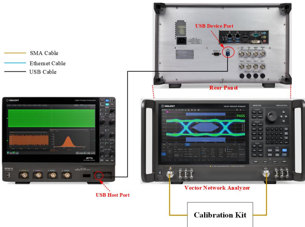
Figure 5-24 Calibration environment for return loss by using Balanced Measure method
