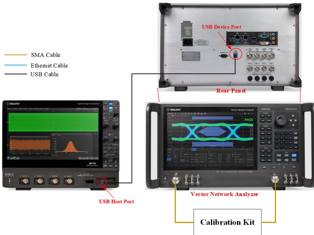
Figure 6-16 Calibration environment for return loss by using Balanced Measure method
